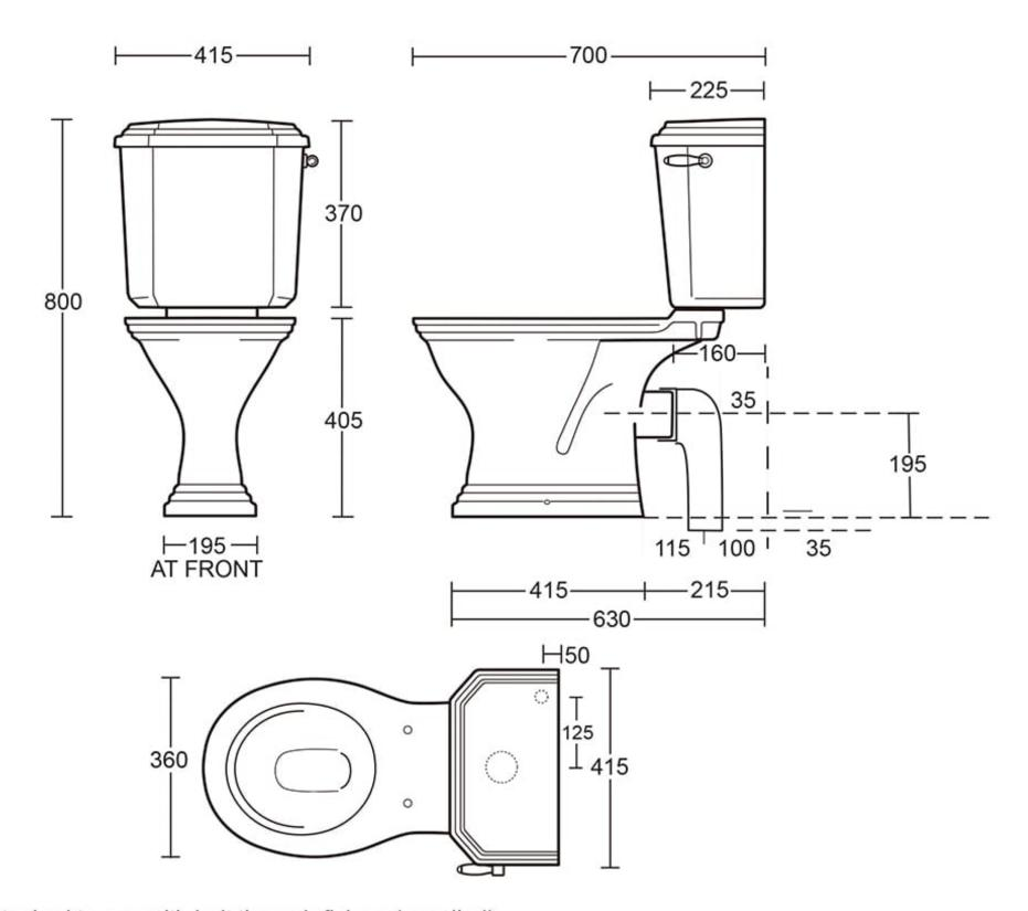
Cistern attached to pan with bolt through fixings (supplied)
